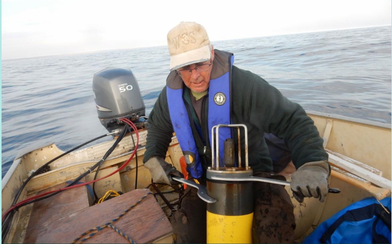
Dr. Steve Insley prepares a sound recorder for deployment in the Western Arctic Ocean. Photo: WCS Canada
